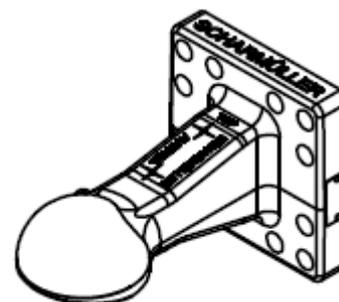
Coupling heads 80 type 80-665901 may only be used in conjunction with the type approved, for mounting suitable draw bars, that are suited for coupling ball couplings 80 according to ISO 24347 and that fulfill the required parameters and allow the required horizontal ( $\pm 60^\circ$ ), vertical and axial ( $\pm 20^\circ$ ) pivoting angles.
